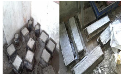
Figure 2 casting of cubes, cylinders and beams
