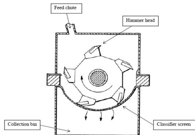
Fig-2 : Mechanical recycling of CFRP cutting conditions.
