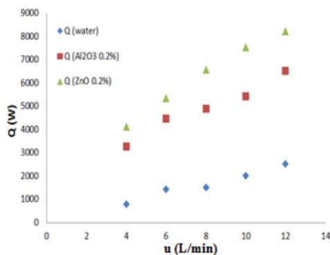
Chart -4: Comparison of heat transfer between the fluids used in the study.
