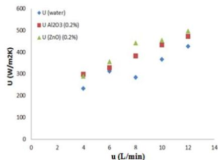
Chart -6: Comparison of overall heat transfer coefficient for the fluids used in study
