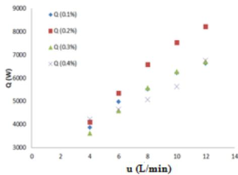
Chart -3: Effect of volumetric concentration on heat transfer of ZNO nano fluid
