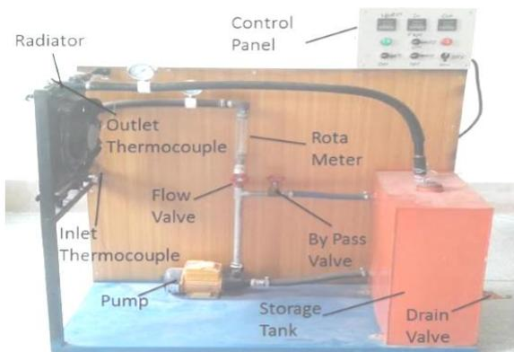
Fig -1: Experimental setup of car radiator
