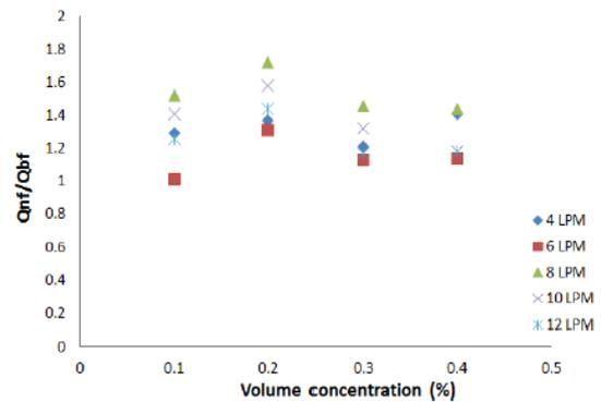
Chart -5: Heat transfer ratio for ZNO with pure water as base fluid at different concentrations
