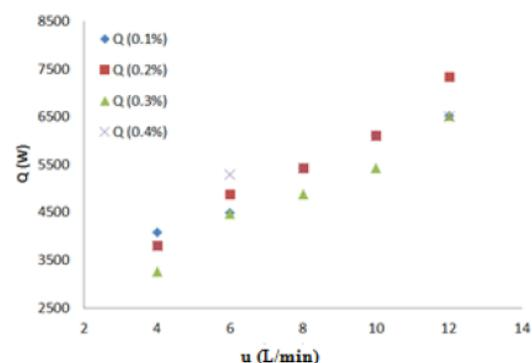
Chart -2: Effect of volumetric concentration on heat transfer of  $AL_2O_3$  nano fluid
