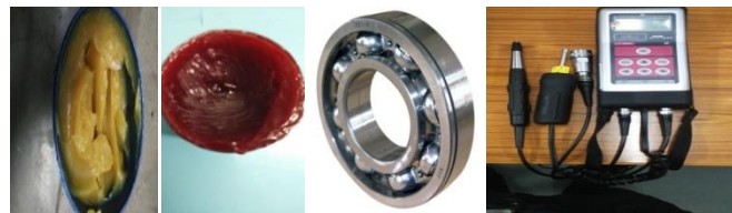
Li grease Ca grease 6206 bearing SPM T30 machine
