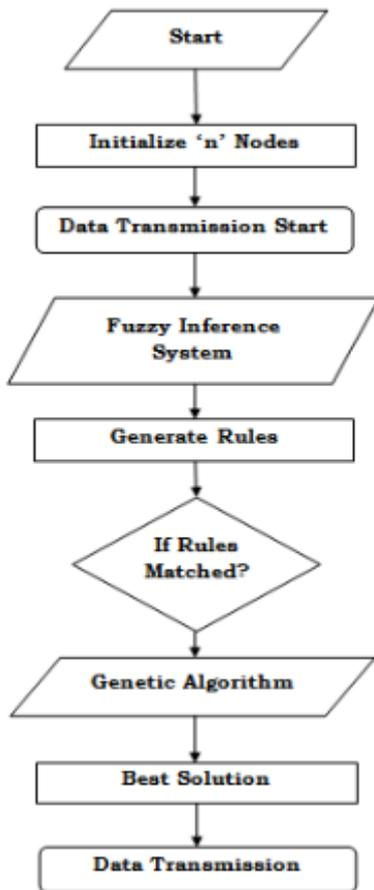
Figure 2: HFGA flow diagram
