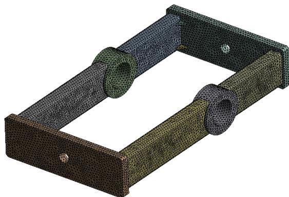
Fig - 5: FE Model of prototype
