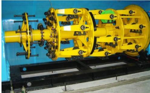
Fig - 1: View representing typical planetary wire stranding Machine
