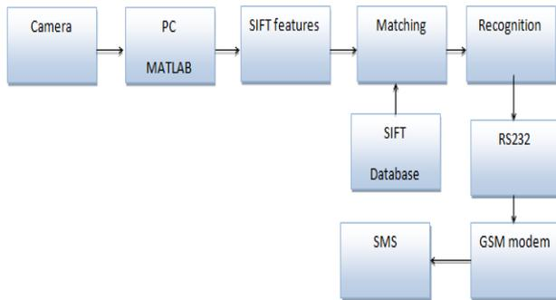
Fig -1: Block Diagram of Face Recognition System
