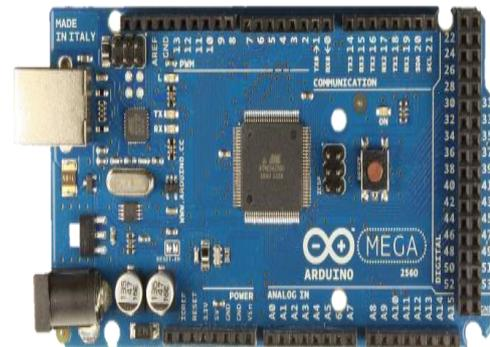
Fig 1 – Arduino MEGA 2560
