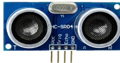
Fig 2 – Ultrasonic sensor HC-SR04
