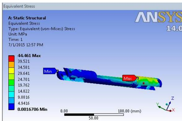
Figure-8: Equivalent stress (von-misses) of rack rod
