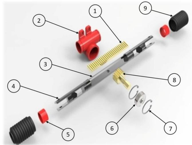
**Fig -1:** Assembly diagram of steering rack and pinion
