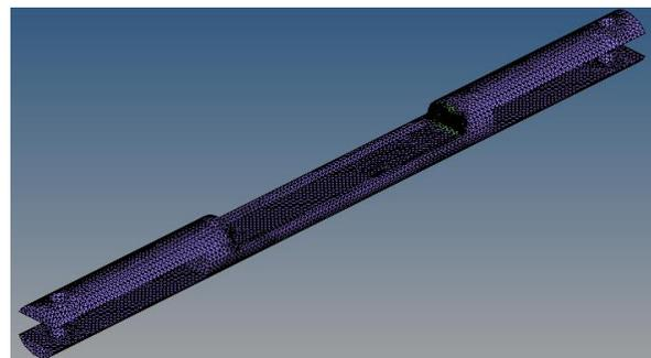
**Figure-5:** Meshed model of rack rod
