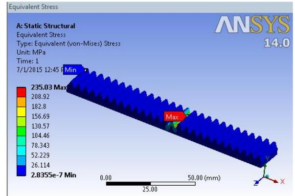
Figure-10: Equivalent stress (von-misses) of rack rod
