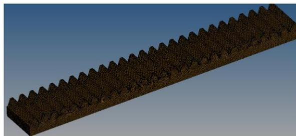
**Figure-6:** Meshed model of rack teeth
