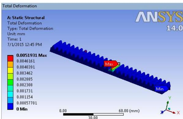
Figure-9: Total deformation of rack teeth
