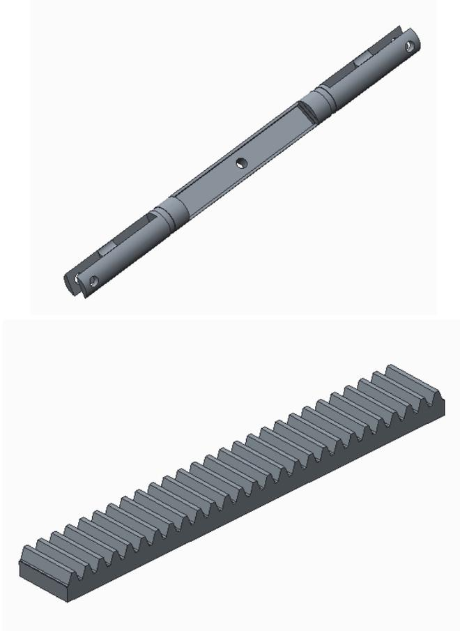
Fig -3: CAD model of Rack rod and Rack teeth
