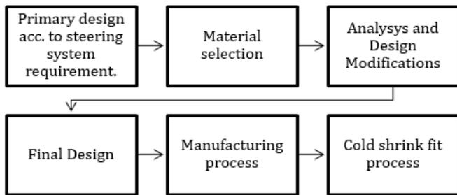
Fig -2: Methodology for design of Composite Rack
