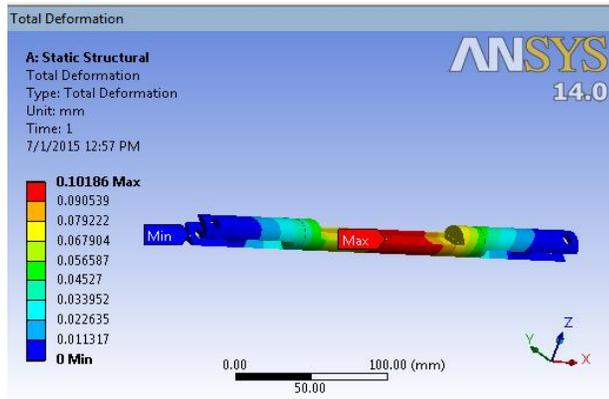
Figure-7: Total deformation of rack rod
