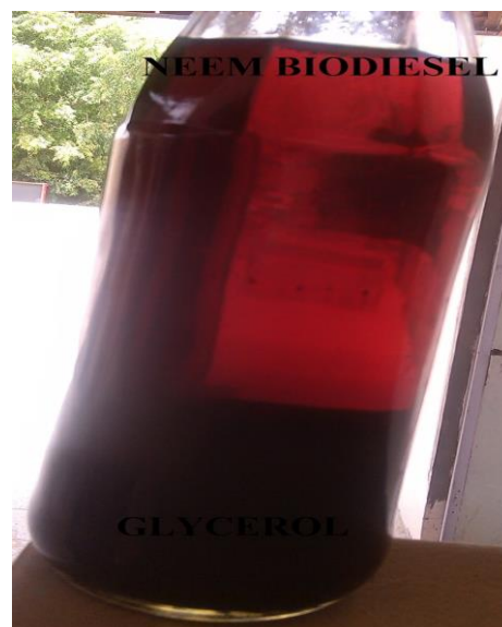
Fig -4: Separation layers of neem biodiesel & glycerol
