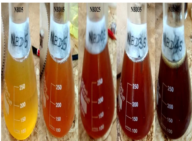
Fig -5: Different blends of neem biodiesel in diesel
