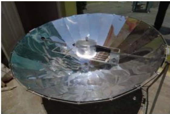
Fig 2 concentrating type of solar cooker[2]
