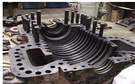
Fig -2: Steam turbine casing
