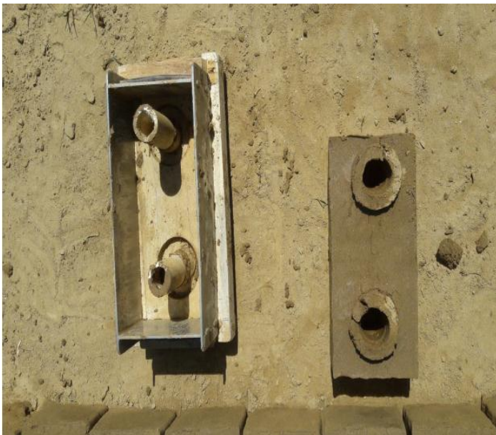
Fig -1: The Mould For Brick Making With A Brick Adjacent To It
