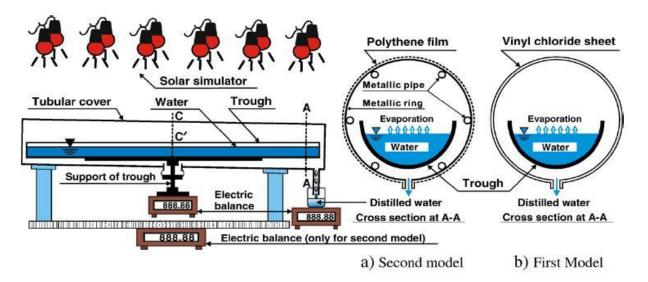
Fig.16. Schematic diagram of a tubular design solar still [32]
