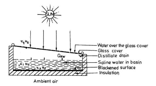
Fig.3. Schematic diagram of a Single Basin Single Slope Solar Still [17]
