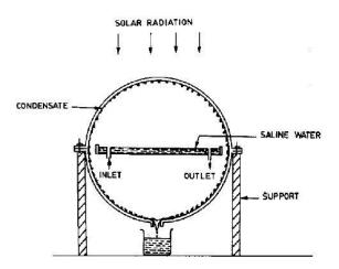
Fig.18. Schematic diagram of a spherical design solar still [35]
