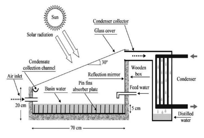
Fig.10. Schematic diagram of a solar still with fins [27]
