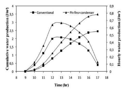
Fig.13. Evolutions of the water production for the conventional still and the still with pin fins absorber and condenser. [27]
