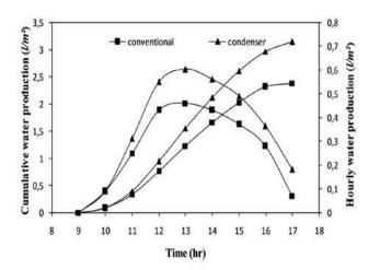
**Fig.11.** Evolutions of the water production for the conventional still and the still with pin fins absorber [27]
