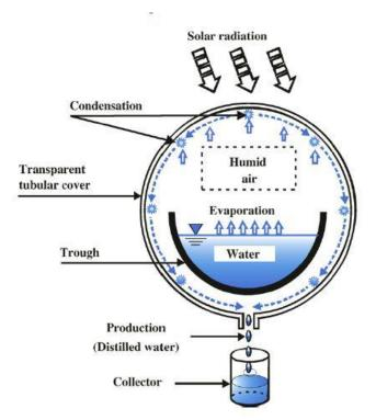
Fig.15. Schematic diagram of a tubular design solar still [32]
