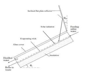
Fig.5. Schematic diagram of a solar still with reflector [20]
