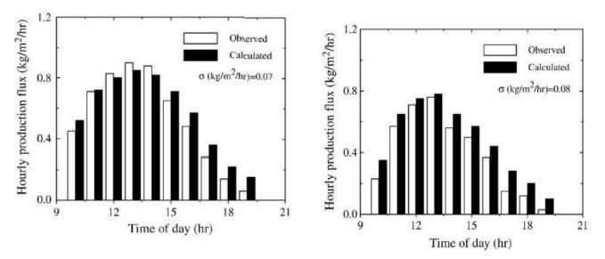
Fig.17. Schematic diagram of a tubular still hourly productivity [32]
