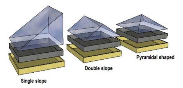
Fig.19. Schematic diagram of a pyramidal design solar still [36]
