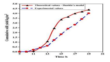
Fig.8 Comparison of theoretical cumulative still yield with the experimental still yield [22]
