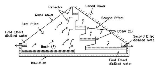
Fig.2. Schematic diagram of passive solar still [13]
