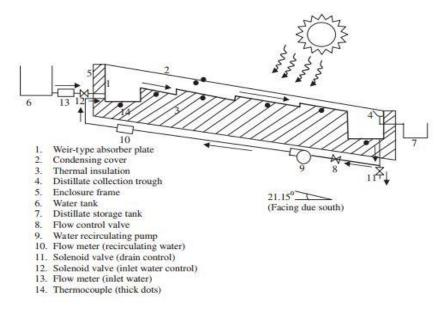
Fig.9. Schematic diagram Weir type solar still [25]
