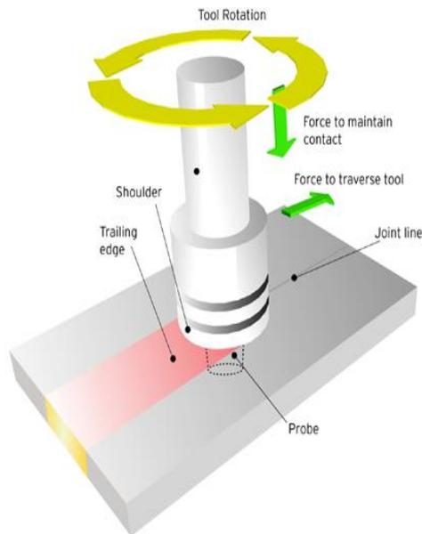
FSW is a solid-state joining process that creates high-quality, high-strength joints with low distortion and is capable of fabricating either butt or lap joints, in a wide range of material thicknesses and lengths.
