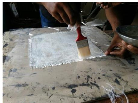
**Fig 1: shows the hand lay-up procedure carried out for Glass epoxy composites.**
