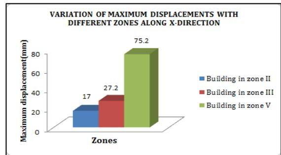
Figure 1: Variation of maximum displacements under different zones along X-direction
