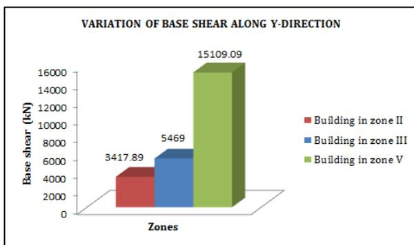
Figure 4: Variation of maximum base shear under different zones along Y-direction
