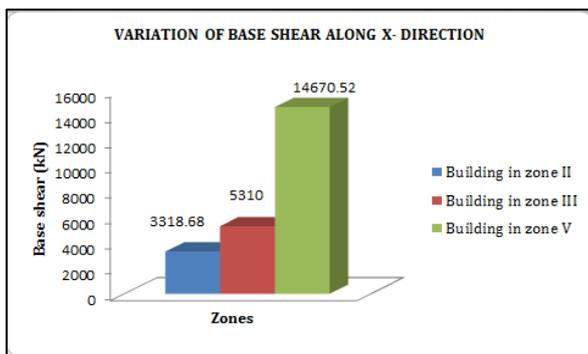
Figure 3: Variation of maximum base shear under different zones along X-direction
