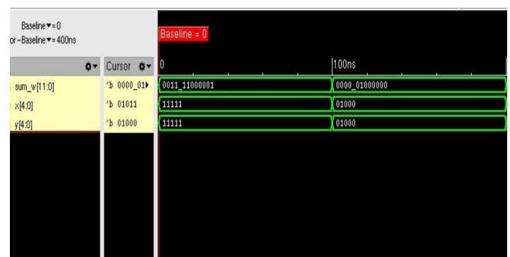
Fig -11: Output waveform of proposed Wallace Tree Multiplier using Carry Save Adder and MUX implementation of Full Adder in binary format
