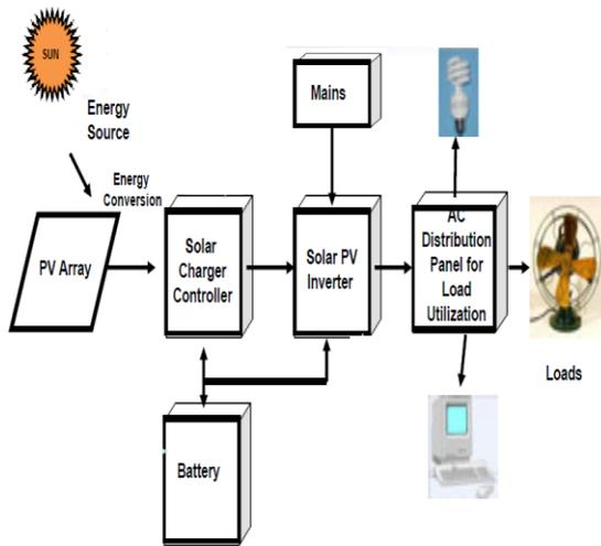
Fig. 2.1: Block Diagram of Off Grid Solar Inverter
