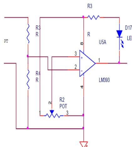
Fig.1: Circuit Diagram of Overvoltage Protection.
