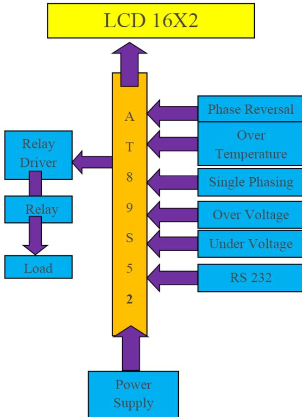
Fig. 5: Block Diagram of System
