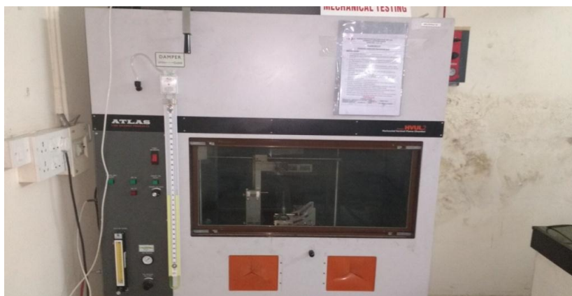
Fig 3. Horizontal and vertical test chamber gas torch
