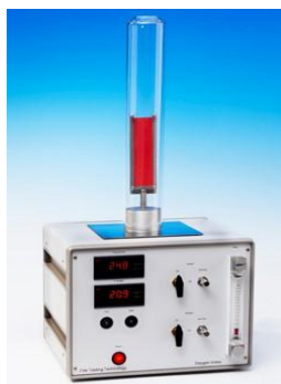
Fig 2. Experimental Set Up Of LOI Test
