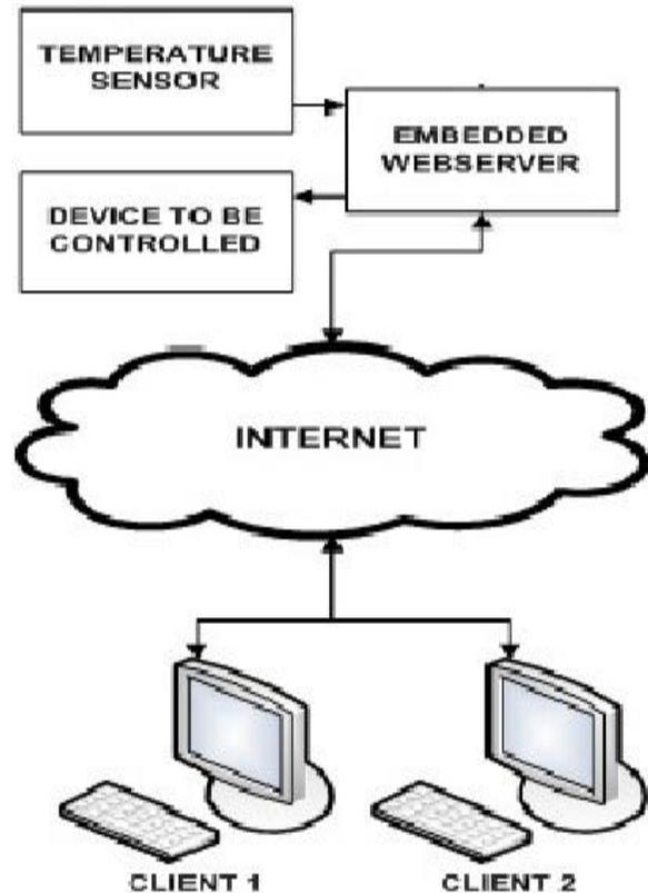
**Fig1- System Architecture of The Proposed Embedded Web Server**
