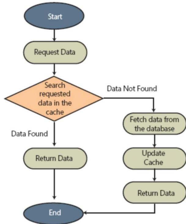
The data can be accessed by client anywhere by using the address of web server. The client can request to server to access the data. If data is found then data is given to client and data is automatically refreshed within a few seconds. If data is not found then it is fetched from database.
