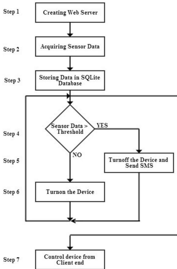
Above flowchart shows design and implementation of web server. The first step is creating the web server address. We acquire the sensory data using that web server address. The data that we have acquired, stored in database. If output of sensor goes above threshold level then control action take place. That is the device will turn off and it will send SMS. If output of sensor does not go above threshold level then it again turn on the device.
