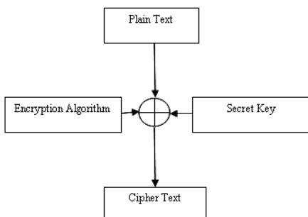
**Fig 3:** Symmetric encryption
