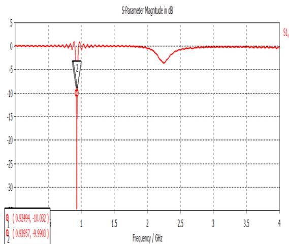
Figure 5 : Return Loss with slots
