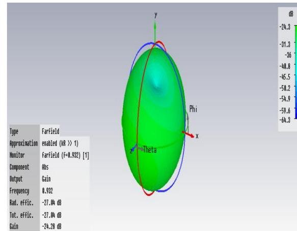
Figure 7: Gain at 0.932GHz
