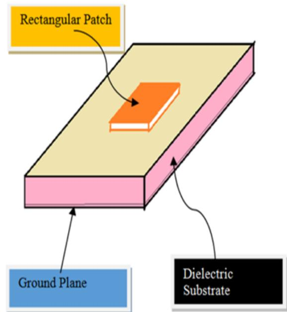
Figure 1: A Basic Rectangular Microstrip Patch antenna
