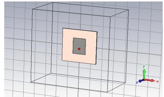
Figure 2: A Rectangular microstrip patch antenna without slots
