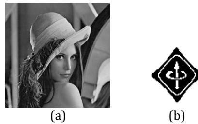
Fig-4: Result against median filter (window size=3x3), (a) Watermarked image (b) Extracted watermark
