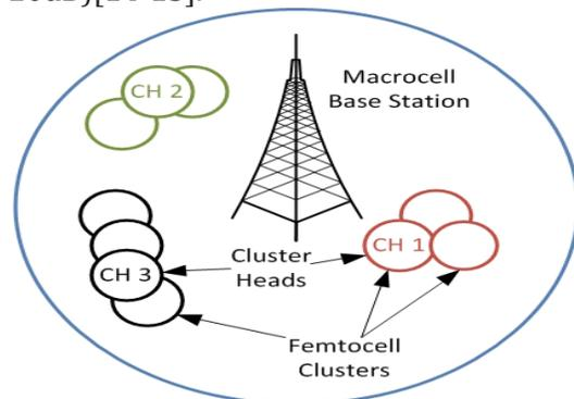
Fig : Clustered femtocell network
