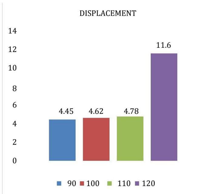
**Chart -1:** Comparison of displacement by variation of alignment of side wall with base slab
