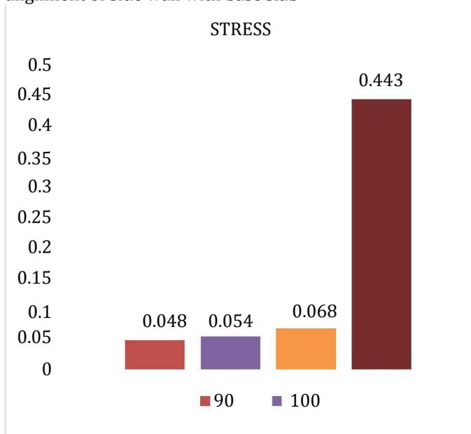
**Chart -2:** Variation of shear stress due to variation of alignment of side wall with base slab
