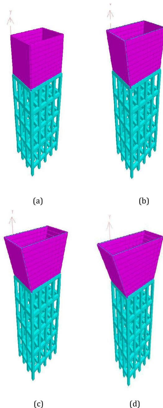
**Fig -1:** Model of elevated water tank by variation of angle of alignment of side wall at angles (a)90° (b)100° (c)110° (d)120°
