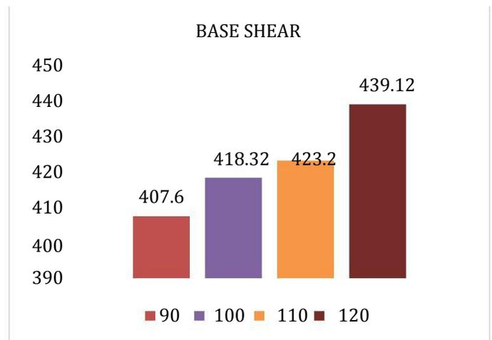
**Chart -3:** Base shear values of elevated water tank by varying the alignment of side wall with base slab
