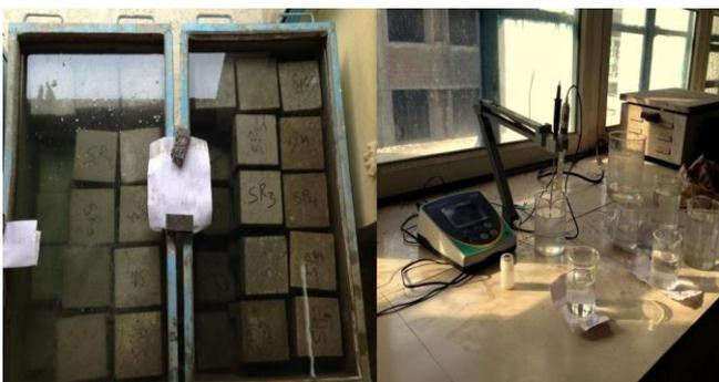
Fig -4: Cubes kept in acid and alkalinity solution and apparatus for measuring pH of solution (pH meter).
