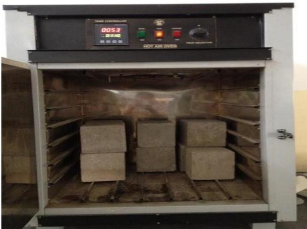
Fig -6: Conditioning and drying of samples in dessicator and oven respectively.
