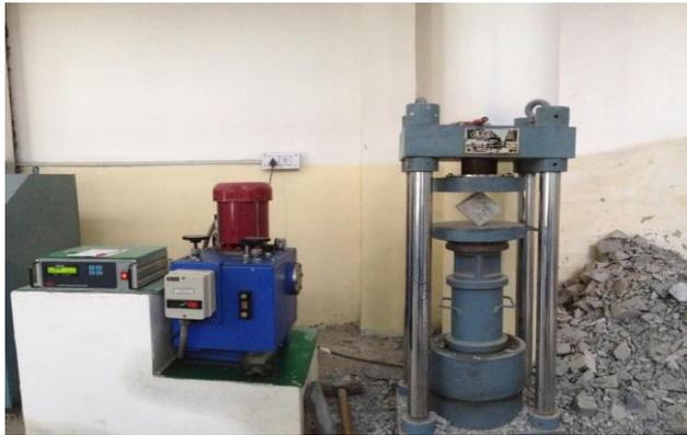
Fig -3: Compression Test Machine
