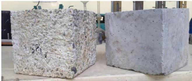
**Fig -7:** Concrete specimens subjected to alkalinity attack, compared with normally cured specimens
