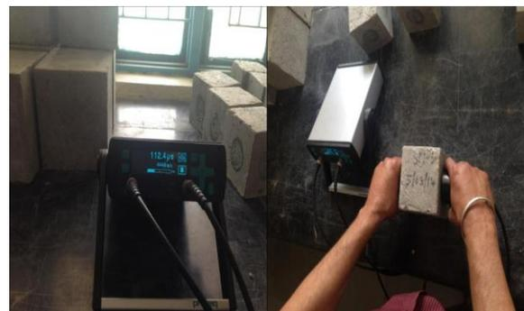
Fig -5: Cubes kept for UPV Test Apparatus
