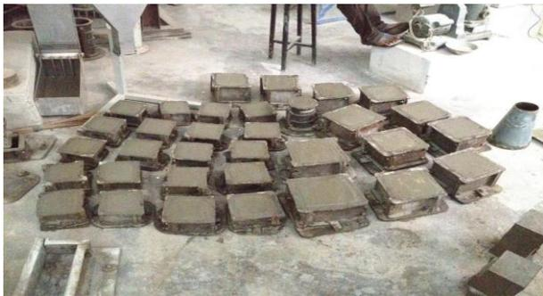
Fig -1: Preparation of Casted Concrete Moulds
