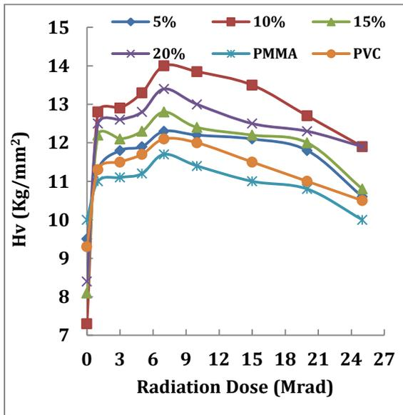
**Fig 1:** Variation of  $H_v$  with various doses of gamma irradiation at 60 g specimen of PVC, PMMA and PVC:PMMA with different wt% of PMMA.
