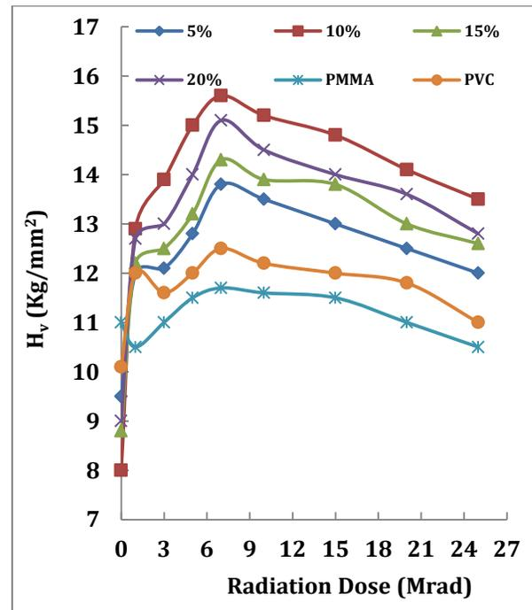
**Fig 2:** Variation of  $H_v$  with various doses of gamma irradiation at 100 g specimen of PVC, PMMA and PVC:PMMA with different wt% of PMMA.
