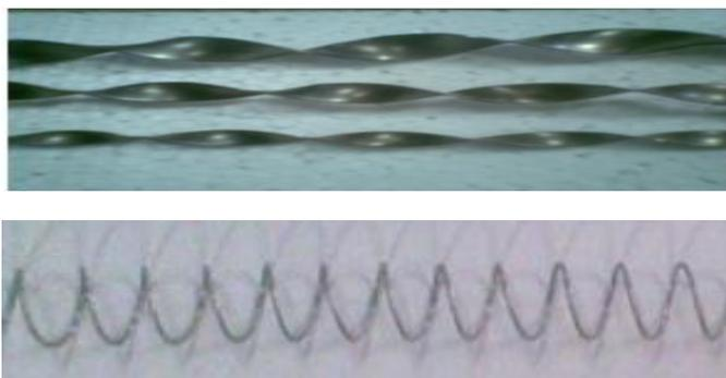
Fig. 6.5 Details Of Twisted Tape And Wire Coil
