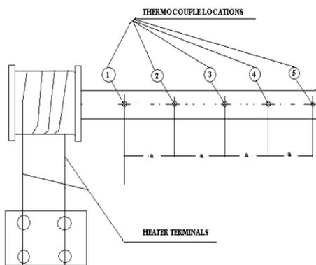
Fig. 7.2 Schematic diagram of pin fin apparatus ( 2 )
