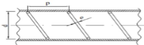
Fig 6.2 Helical Wire Coil Fitted Inside A Smooth Tube
