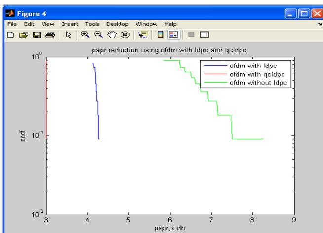
Fig. 5. Plot PAPR reduction in OFDM system with BPSK modulation.
