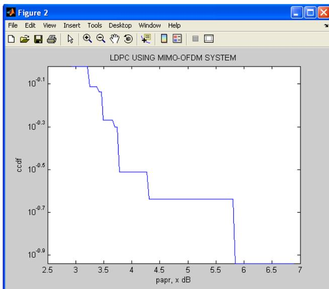
Fig. 4. Plot for PAPR reduction MIMO-OFDM system using LDPC codes.
