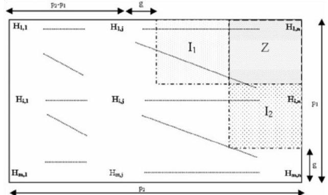
Fig 2: The parity check matrix H
