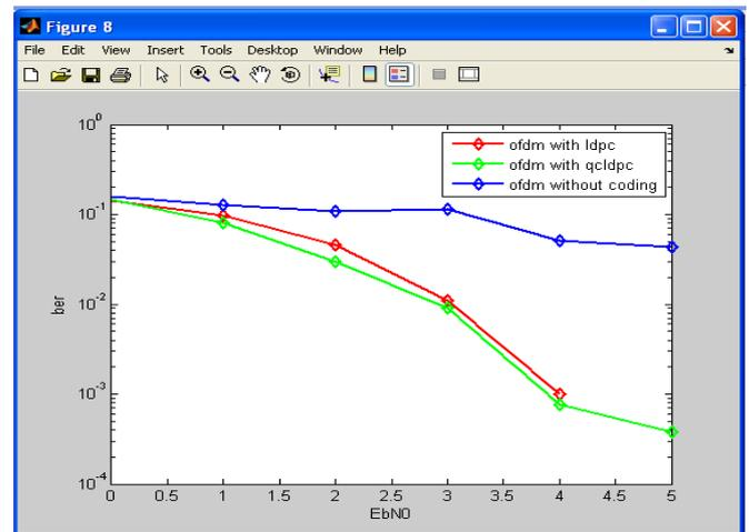
Fig. 6. BER plot for OFDM without coding, LDPC codes, and QCLDPC codes
