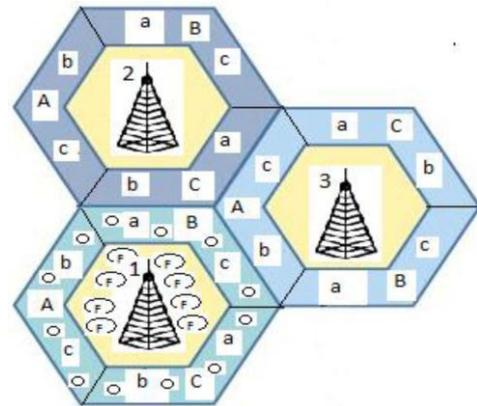
Fig -1: Femtocells deployment in Macrocells
