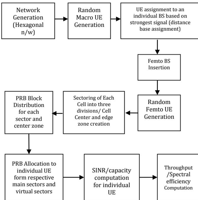
**Fig-2:** Equal distribution of power for improving system capacity through on request channel allocation
