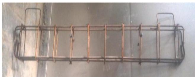
**Fig -3:** Reinforcement details of Beam
