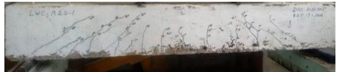
**Fig -9:** Crack Pattern of M20 LWC Beam #1
