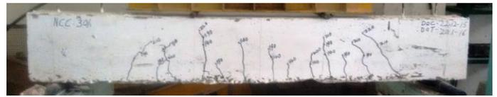
**Fig -8:** Crack Pattern of M30 NCC Beam #1
