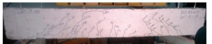
**Fig -10:** Crack Pattern of M30 LWC Beam #1
