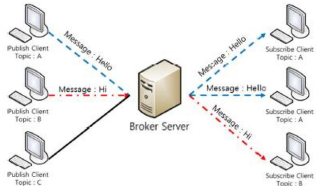
Figure 2. MQTT Message Transmission Process
