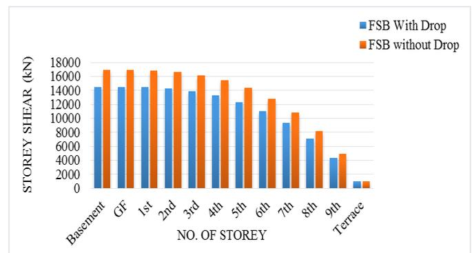
**Chart 13:** Storey Shear verses Number of Storey for FSB with and without Drop for Zone V
