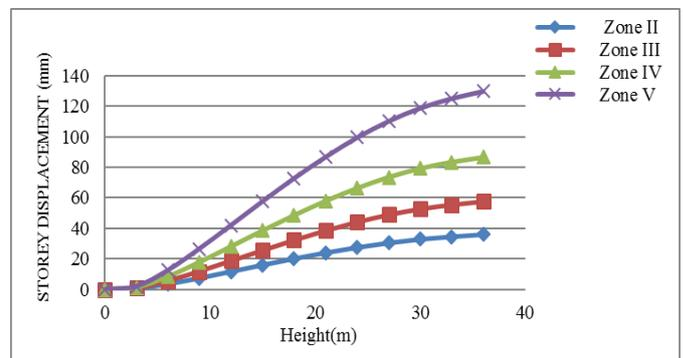
Chart 1: Storey Displacement verses Height for Flat Slab with Drop
