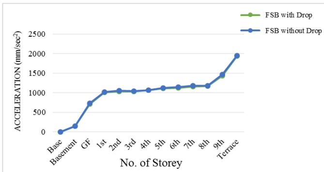
**Chart 14:** Acceleration versus Number of Storey for FSB with and without Drop for Zone V
