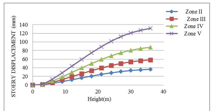
**Chart 6:** Storey Displacement versus Height for flat slab without Drop
