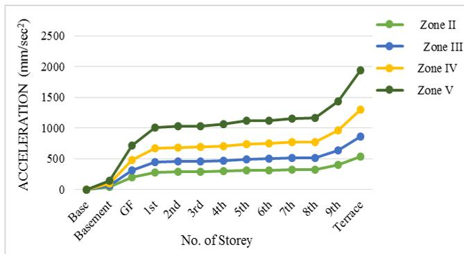
**Chart 5:** Acceleration versus Number of Storey for Flat Slab with Drop
