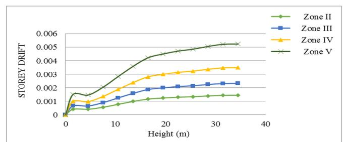
**Chart 7:** Storey Drift versus Height for Flat Slab without Drop
