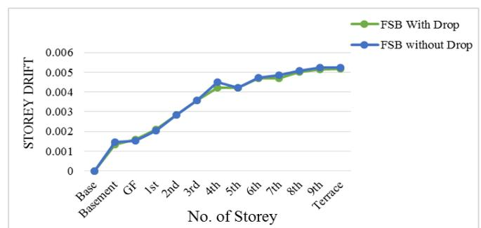
**Chart 12:** Storey Drift verses Number of Storey for FSB with and without Drop for Zone V
