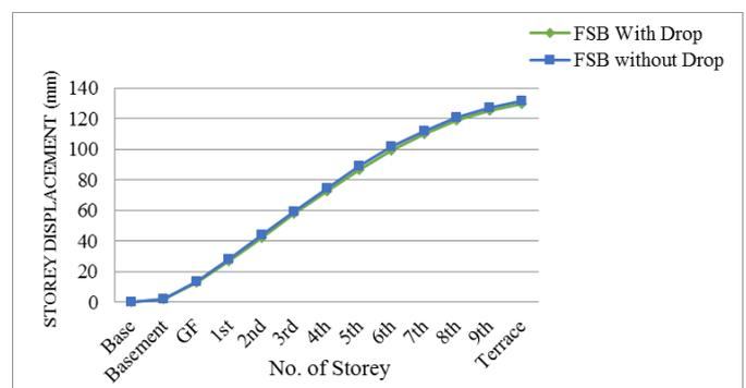
**Chart 11:** Storey Displacement verses Number of Storey for FSB with and without Drop at Zone V
