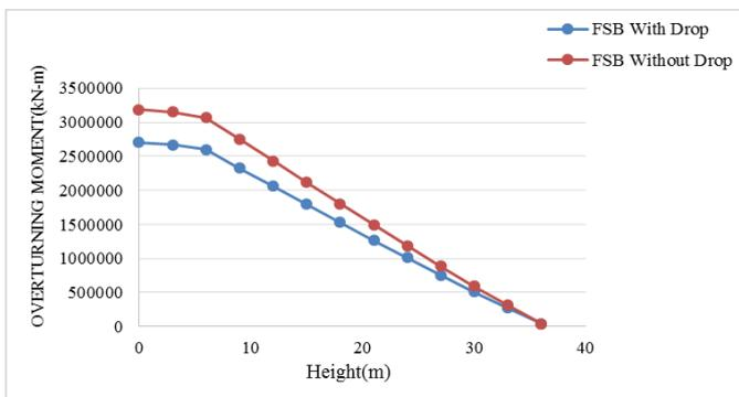
**Chart 15:** Overturning Moment versus Height for FSB with and without Drop for Zone V
