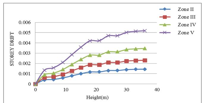
Chart 2: Storey Drift verses Height for Flat Slab with Drop
