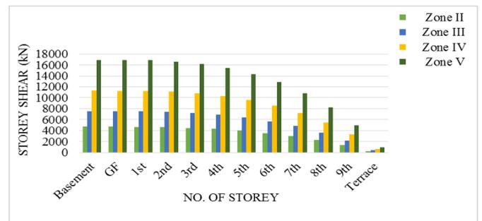
**Chart 8:** Storey Shear versus Number of Storey for Flat Slab without Drop
