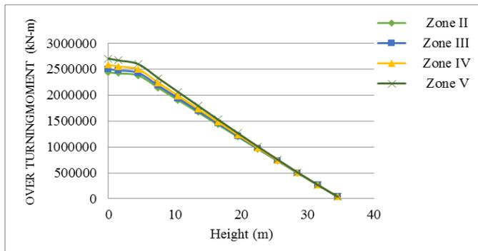
**Chart 3:** Overturning Moment versus Height for Flat Slab
