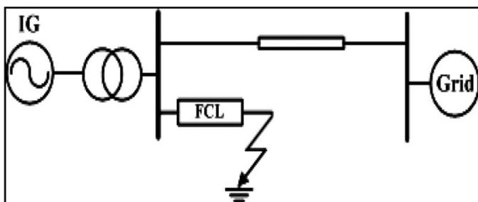
**Fig.2.3 Equivalent circuit of power system.**
