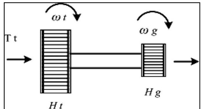
Fig. 2.2 Two mass model of wind turbine train
