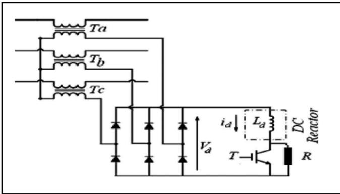
Fig.1.1 Bridge-type FCL with discharging resistor.
