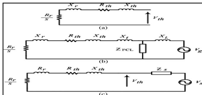
**Fig.2.4 (a) Steady-state equivalent circuit of induction generator. (b) Equivalent circuit of system with FCL during fault. (c) Equivalent circuit of system seen from IG terminals.**
