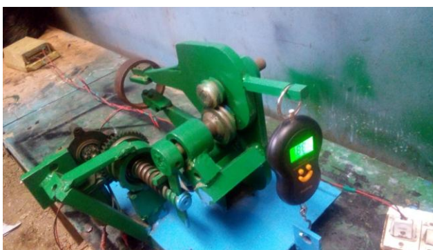
Fig- 4.1: Actual Experimental Set up Internal Expanding Jaw Gripper System
