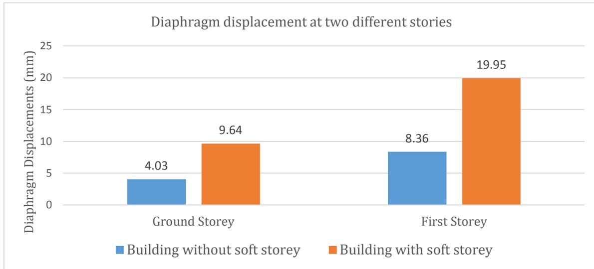
It is observed from Graph 1 that diaphragm displacements for building with soft storey is more than building without soft storey at both ground and first storey level. This is partially because of 2.5 times magnification factor for soft storey building.
