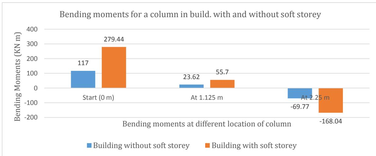
Bending moments for a column in building with soft storey is higher than building without soft storey as soft storey is designed for 2.5 times magnification factor. Modification of load combinations caused by this factor induces more forces and moments in beams, columns and shear walls.
