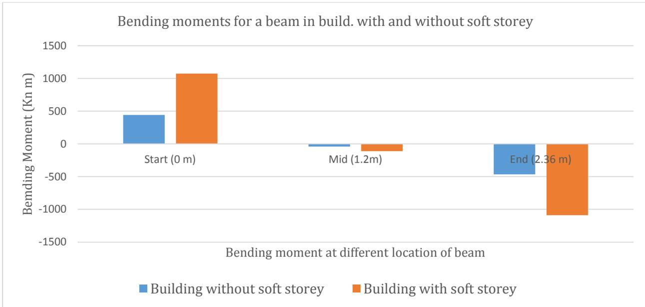
Bending moments for a beam in building with soft storey is higher than building without soft storey as soft storey is designed for 2.5 times magnification factor. Modification of load combinations caused by this factor induces more forces and moments in beams, columns and shear walls.
