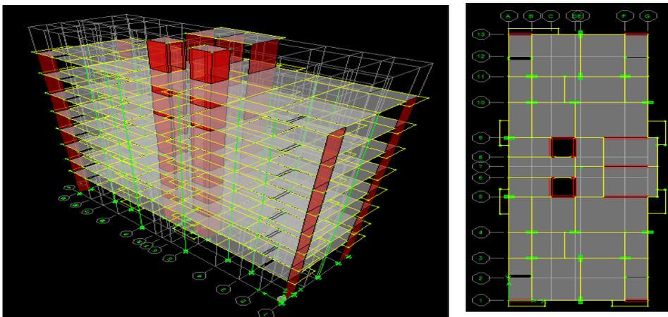
Figure 1 – 3 D view of building with basement, ground and 6 storeys along with plan of the building
