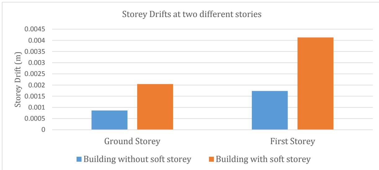
Storey drift is higher for building with soft storey at ground and first storey when compared to building without soft storey which can be seen from graph 2. This is partially because of magnification factor of 2.5 applied in building with soft storey.
