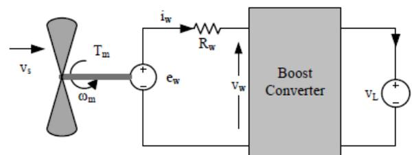
Figure (2) A simplified wind generator system
