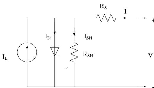
Figure (3) Equivalent circuit of a solar cell.
