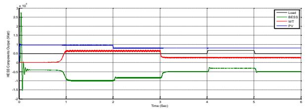
Figure (13) Output power of different components of Hybrid power system
