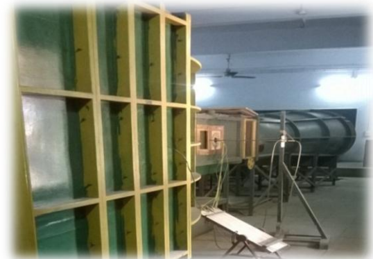
Fig 2.2: Experimental set-up of open air circuit sub-sonic wind tunnel
