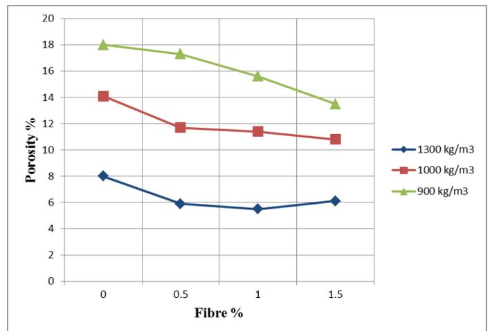
Fig -3 Deviation in porosity with fibre %
