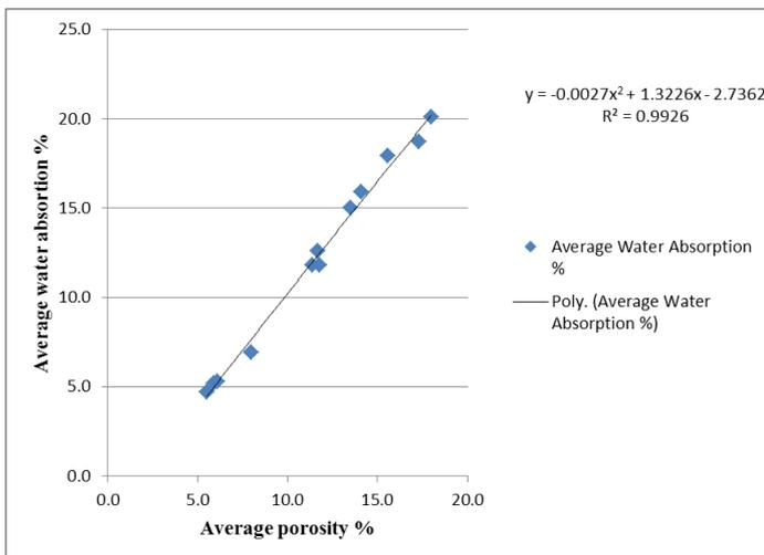
Fig-5 Correlation between avg water absorption with avg porosity
