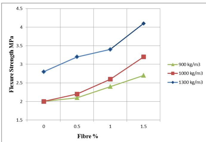
Fig-6 Deviation in flexure strength with fibre %
