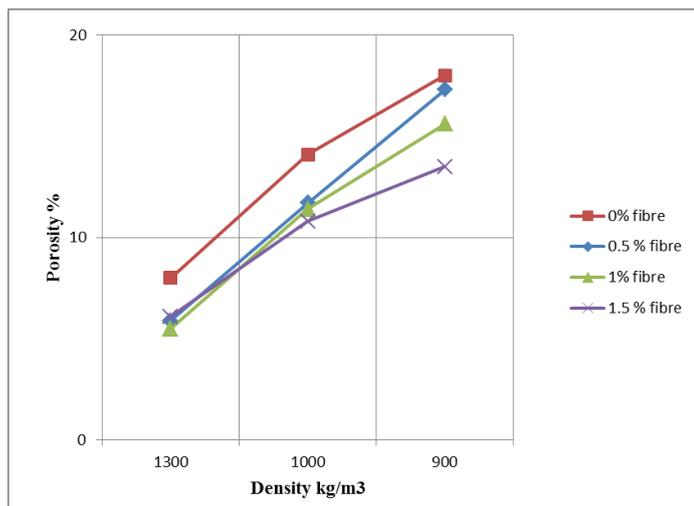
Fig -2 Deviation in porosity with density
