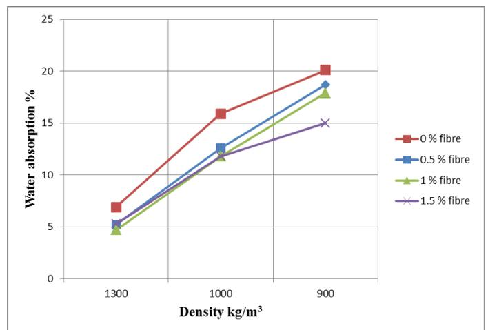
Fig -4 Deviation in water absorption with density
