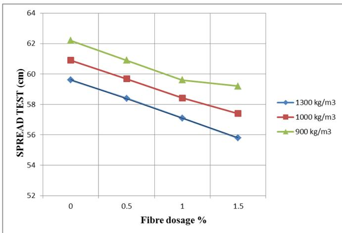
Fig -1 Deviation of Spread test value with fibre content
