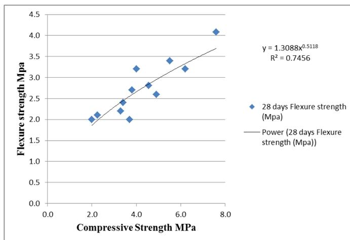
**Fig -8** Correlation between compressive strength and flexure strength
