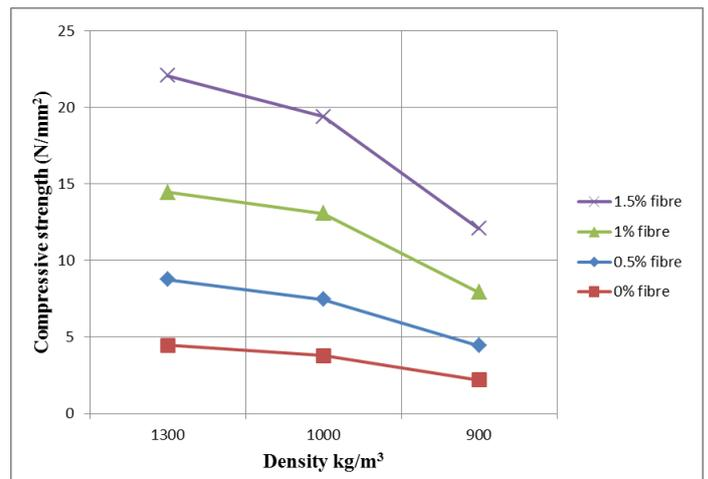
Fig-7 Deviation in Compressive strength with density
