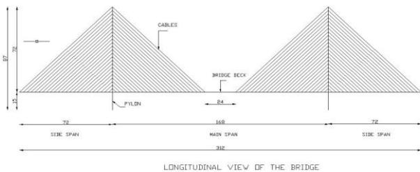
Fig 2 Longitudinal Section of Cable Stayed Bridge
