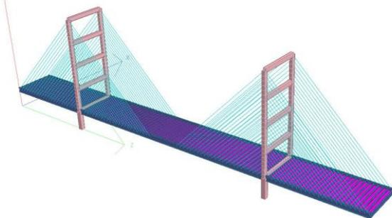
Fig 3 STAAD pro 3-D Model of Two Planes Cable Configuration
