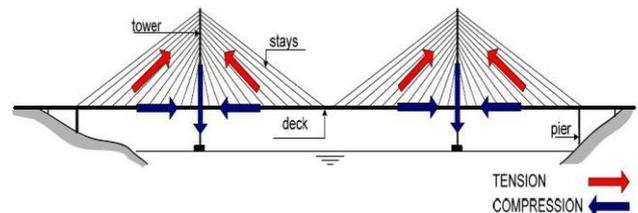
**Fig 1 Figure Showing the Behaviour of Cable Stayed Bridge**
