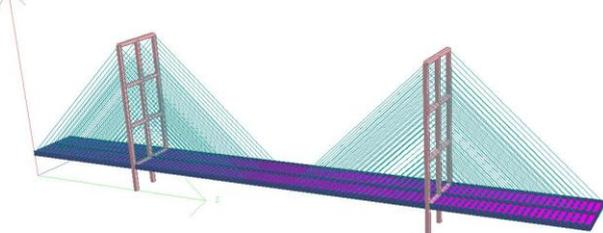
Fig 4 STAAD pro 3-D Model of Three Planes Cable Configuration
