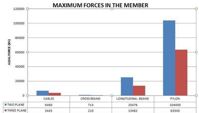
Chart-1: Comparison of Maximum Forces in 2planes and 3planes Cable Configuration of Cable Stayed Bridge.
