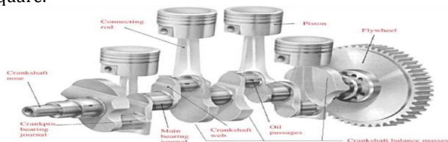
Fig. 1.1 Ordinary crankshaft with principle diary that backing the crankshaft in the motor square
