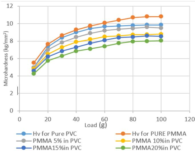
**Fig.(1)** variation of H<sub>v</sub> with load at various weight % of PVC : PMMA polyblend
