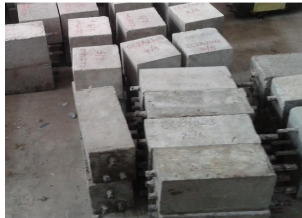
Fig. 1: Corrosion test specimens and cubes
