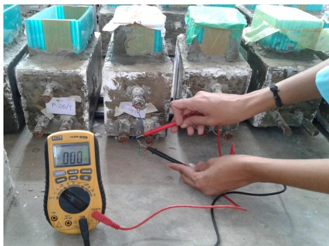
Fig. 2: Macrocell corrosion test set up showing voltage measurement
