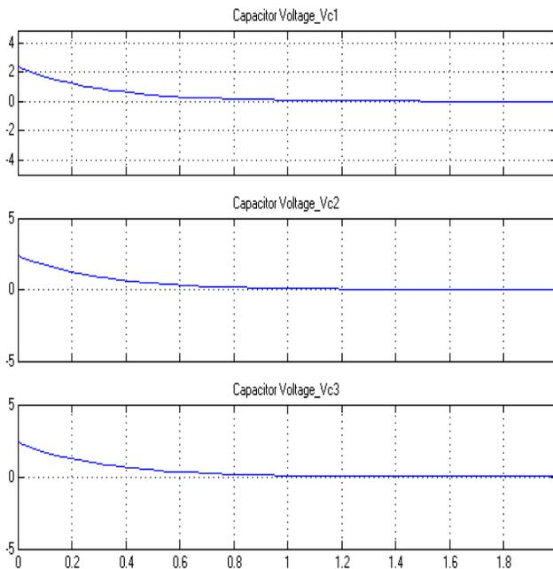
Fig.8. Voltage across capacitors with decreasing waveform.
