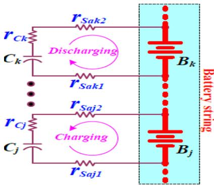
Fig.3. State circuit of new SC equalizer during the phase  $\Phi_a$
