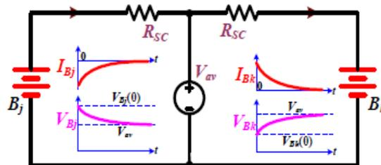
Fig.6. Equivalent circuit of the voltage balancing process.
