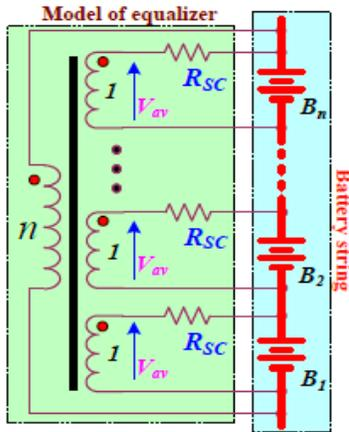
Fig.5. Model of series-parallel SC equalizer
