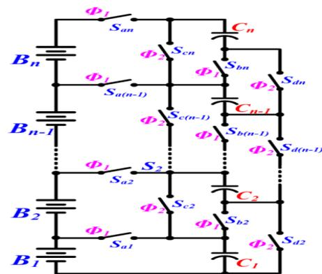
Fig.1. Voltage equalization system implemented by series-parallel switched-capacitor converter
