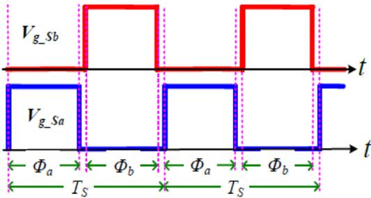
Fig.2. Control signals and time slots of SC equalizers.
