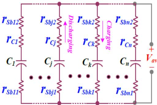
Fig.4. State circuit of new SC equalizer during the phase  $\Phi_b$ .
