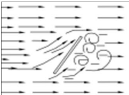
Fig -11: pressure zone around barrier [5]
