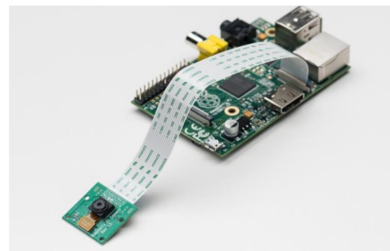
Raspberry Pi with Pi camera
