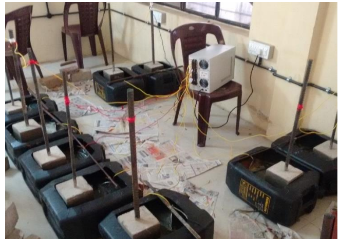
Fig -1: Accelerated corrosion setup
